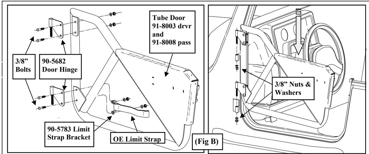
**Step 6:** Carefully install the door assembly onto the vehicle hinges. (Fig B)
