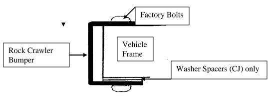
**<u>Step 3:</u>** Tighten all hardware at this time. Installation is now complete.
