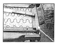
7. Fasten slider to the new seat using the 4 Bolts saved from Step 5.
